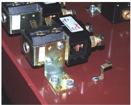
Secure both contactor with 2ea. Scr-Hex(3400315) and 2ea. Nut-Hex(3400172). Tighten with 5/16 wrench and 3/8 wrench.
