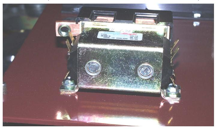
Attach Resistor(3311019) with 2ea. Scr-Hex(3400315) and 2ea. Nut-Hex(3400172). Tighten with 5/16 wrench and 3/8 wrench.
