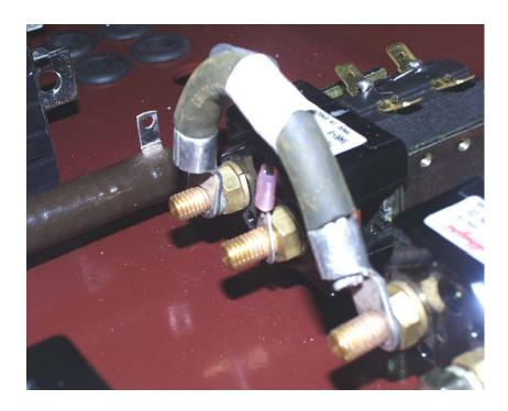
Place Resistor(3311020) and Cable(3311441)onto Contactor as shown.
