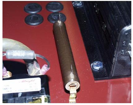
Attach 2ea. Mnt(3311421) with 2ea. Scr-Pan(3400045) and 2ea. Nut-Hex(3400082). Tighten with flathead screwdriver and 11/32 wrench. Attach Resistor(3311567) as shown.
