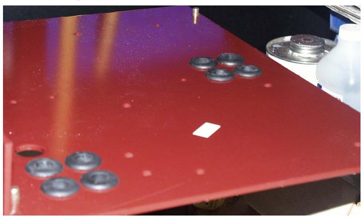
Insert 8ea. Grommet(3311564) into Plate(3311311) as shown.
