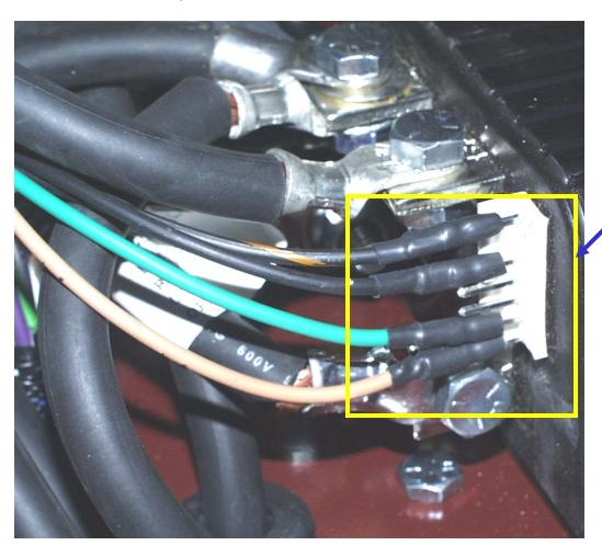
Attach male end to wires and crimp to fit. Apply heatshrink as shown. **REFER TO WIRING DIAGRAM.**
